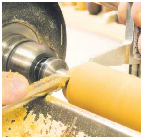
▲ Pic.17 The stem is mounted between centres using a small Stebcentre. The spigot on the bottom has to be a really tight fit so use Verniers to gauge the right diameter
